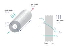
A student assignment with results memorandum evaluates the knowledge and understanding of the students using either hand calculations or Flownex® as software tool. The exercise expects the student to calculate and compare the air side wall surface temperature of both the plane wall and tube scenarios using the same specified wall thickness.
