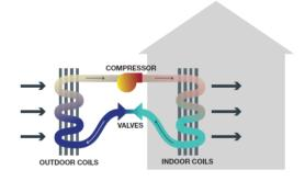
A student assignment with results memorandum evaluates the knowledge and understanding of the students using either hand calculations or Flownex® as software tool. The exercise expects the student to calculate the pressures and temperatures of a basic heat pump system using a pump, valve and specified heat transfer requirement.
