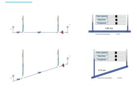
The Flownex® SE network dynamically illustrates the effect of pipe roughness and flow velocity on the energy and hydraulic grade line. The example uses a short pipeline section with an elevation difference between the inlet and outlet (that holds pitot tubes and stand pipes) that indicates the pressure difference.
