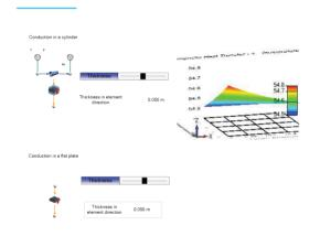
The Flownex® SE network with graphical interface dynamically illustrates the difference between plane wall and cylindrical wall heat transfer with varying wall thickness. The example uses a heat transfer element and pipe combination which either model a tube or plane wall with water flowing on the one side and air over the other.
